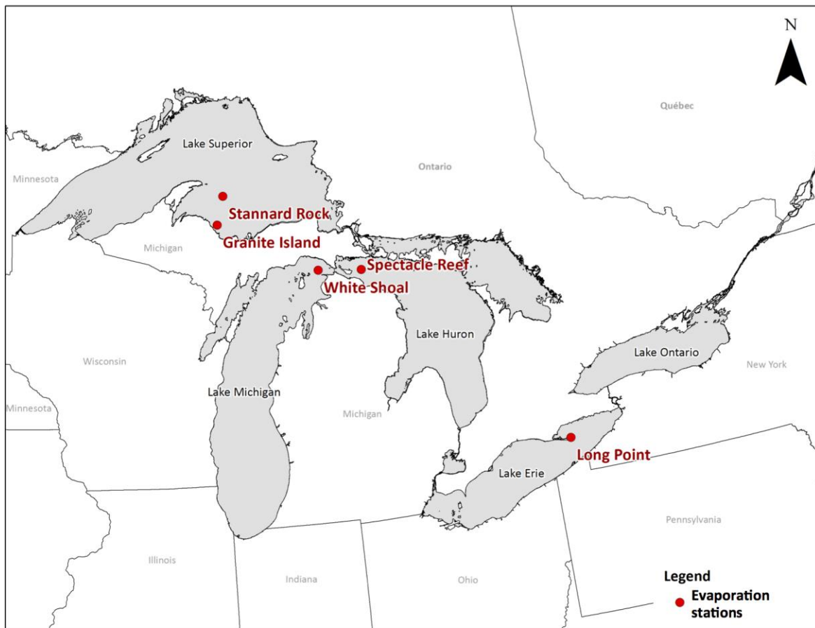
Figure 2. Map showing the new network of evaporation monitoring stations on the Great Lakes. As of November 2013, a total of five stations are in operation, with additional stations planned for the future (funding permitting). All five sites employ the full suite of meteorological instruments that are needed for applying the eddy covariance technique.
